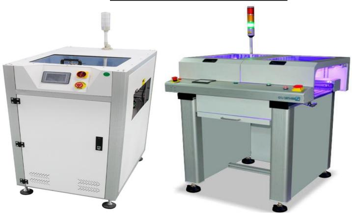
SMLC Provide the conveyorized UV Inspection chamber. Which length is approx. 1/2 meter.
