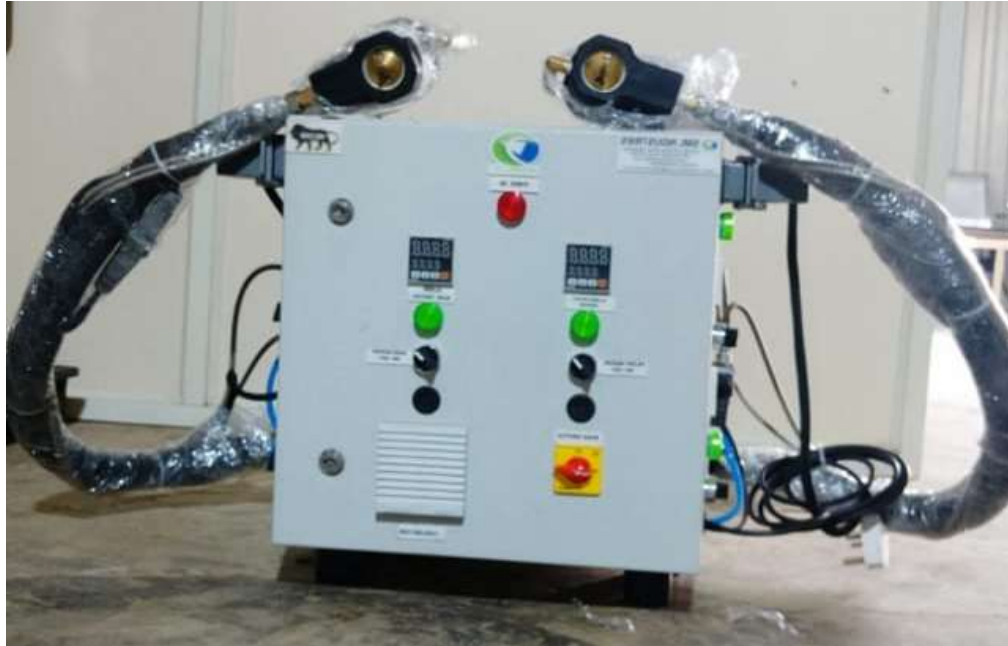
Dual output hot melt dispensing machine with heated hose
